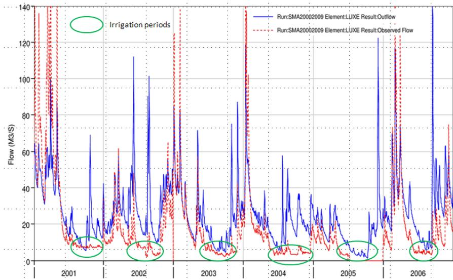
**Figure 4.** HMS model calibrated for wet periods showing the impact of summer irrigation on the river flow (in red : measurements, in blue: the HMS model without irrigation which is calculated in ExtendSim)
