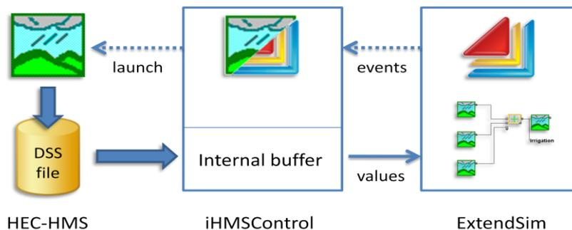
**Figure 2.** HEC-HMS and ExtendSim interface with iHMScontroler to access to the DSS database and provide hydrological forcing values and to launch new run of HMS in batch mode with modified parameters
