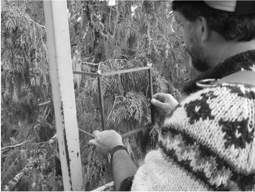
Fig. 2. Subplot frame (25 cm \times 25 cm \times 25 cm) used for selecting sample foliage. For the scale-leaved western red cedar, the length (S) of foliated stems was divided by 10 and then 10 fronds were selected, each S/10 cm apart along stems.
