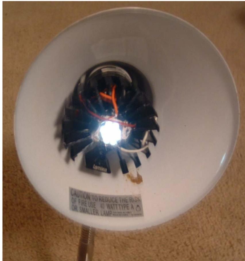
**Figure 6-19 Final Results - The 11.3 V Lamina LED Lit Up**
