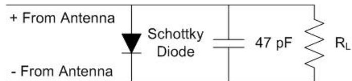
**Figure 4-2 Initial Rectifying Circuit Schematic**
