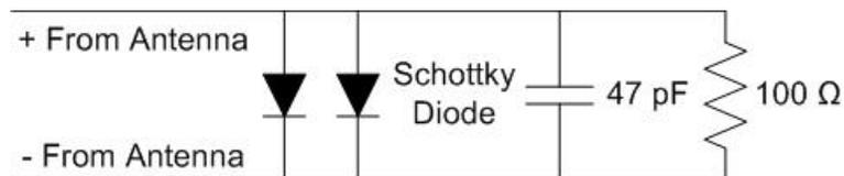
**Figure 6-2 Trial #2 Schematic**
