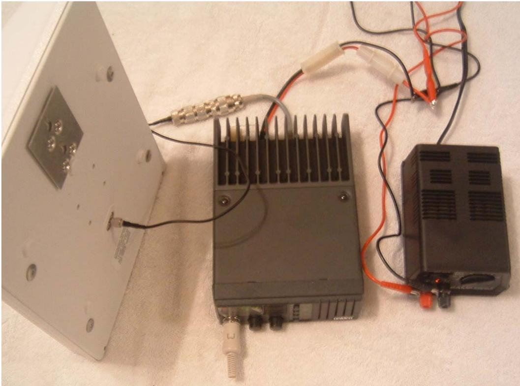
**Figure 4-1 The Transmitting Antenna, Trunking Radio, and Power Source**
