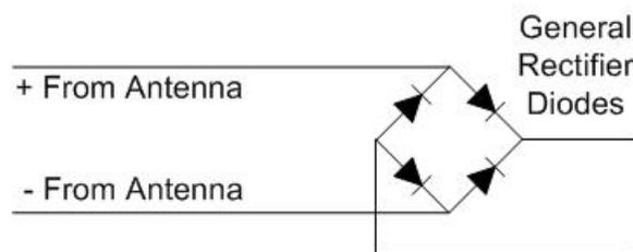
**Figure 6-11 General Rectifier Diode Trial #10 Schematic**
