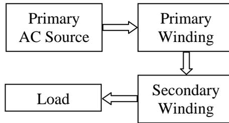
**Figure 2-1 Components of an Inductive Power Transfer System (Stielau 2000)**
