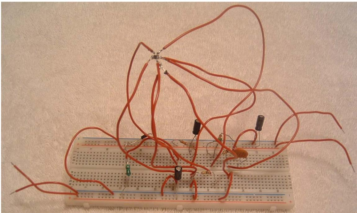
**Figure 6-17 Picture of the Voltage Boost Circuit**
