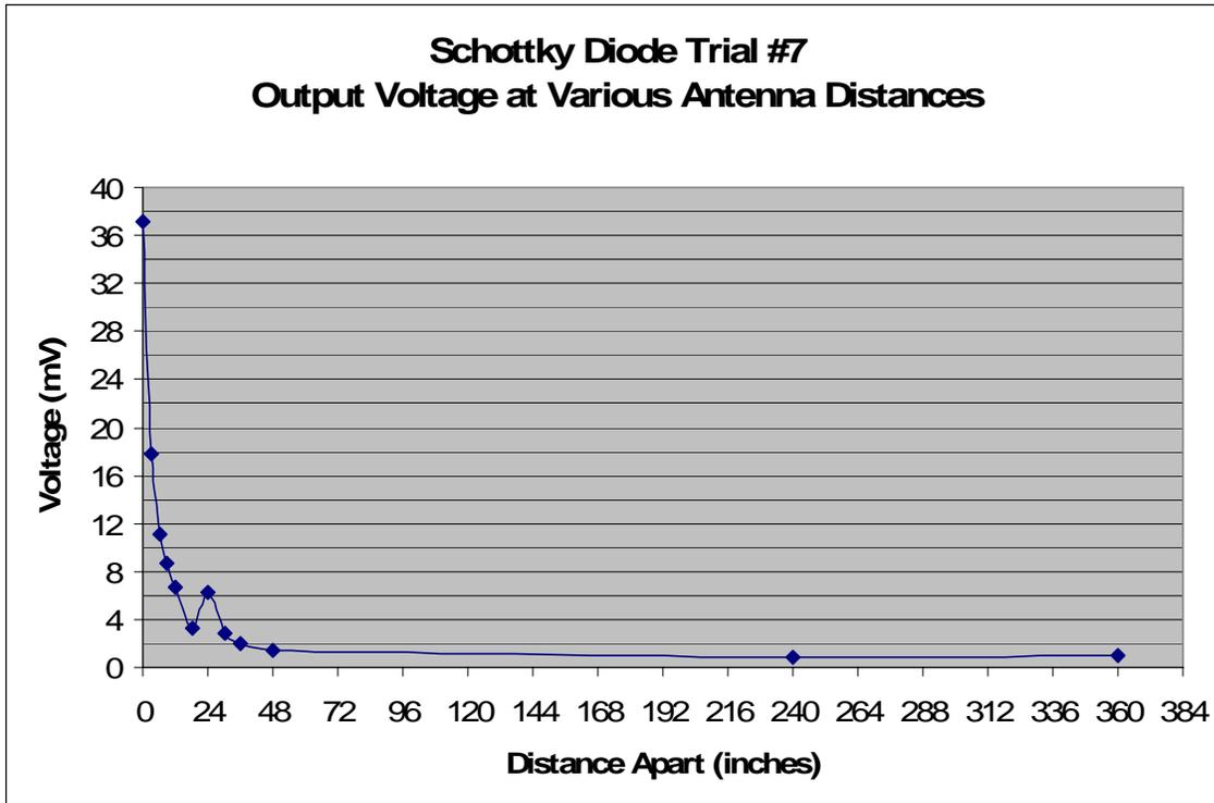
**Figure 6-8 Trial #7 Output Voltage**
