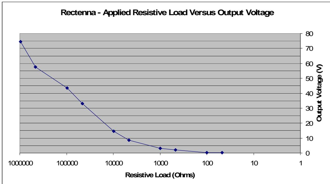
Figure 6-14 Output Voltage with Varying Resistive Loads
