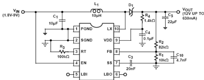
Figure 6-15 Voltage Boost Circuit (Intersil 2005)
