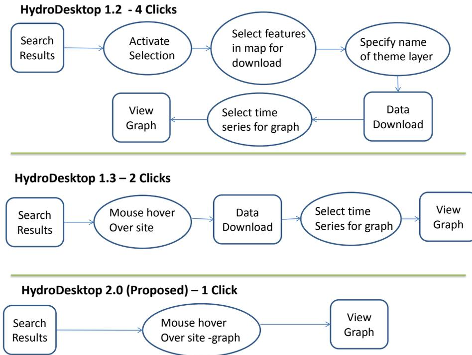
**Figure 5.** Number of steps required from showing search results in a map to displaying time series in a graph. The ellipse represents a required click operation. The current version of HydroDesktop has reduced the number of required steps, but a further reduction (automatic on-demand data download) is suggested.
