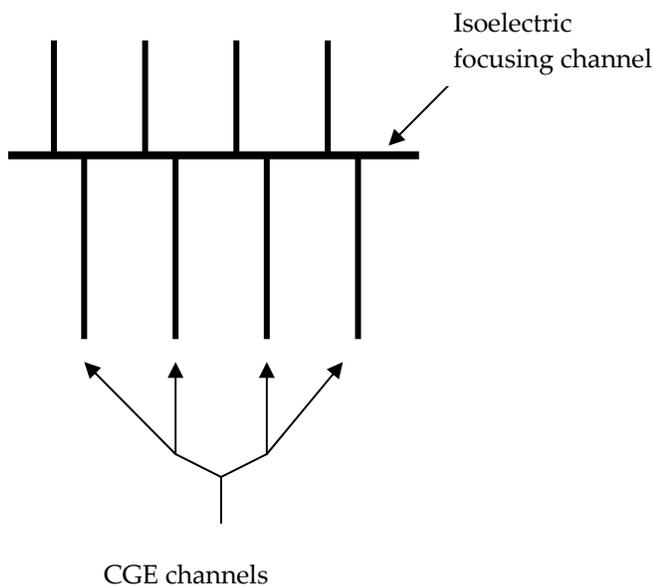
**Figure 4.2.** Schematic of a 2-D (IEF and CGE) microfluidic device.
