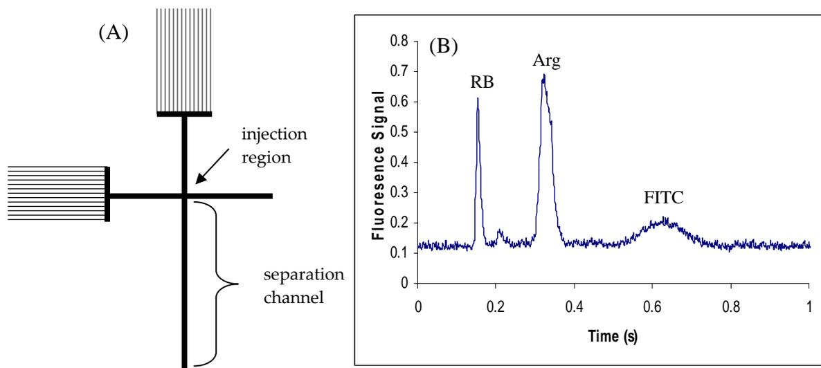
**Figure 4.4.** (A) Device layout for electroosmotically pumped chromatography. Chromatogram of rhodamine B (RB) and FITC-arginine (Arg) obtained at 850 V/cm in a device whose design is shown in (A).
