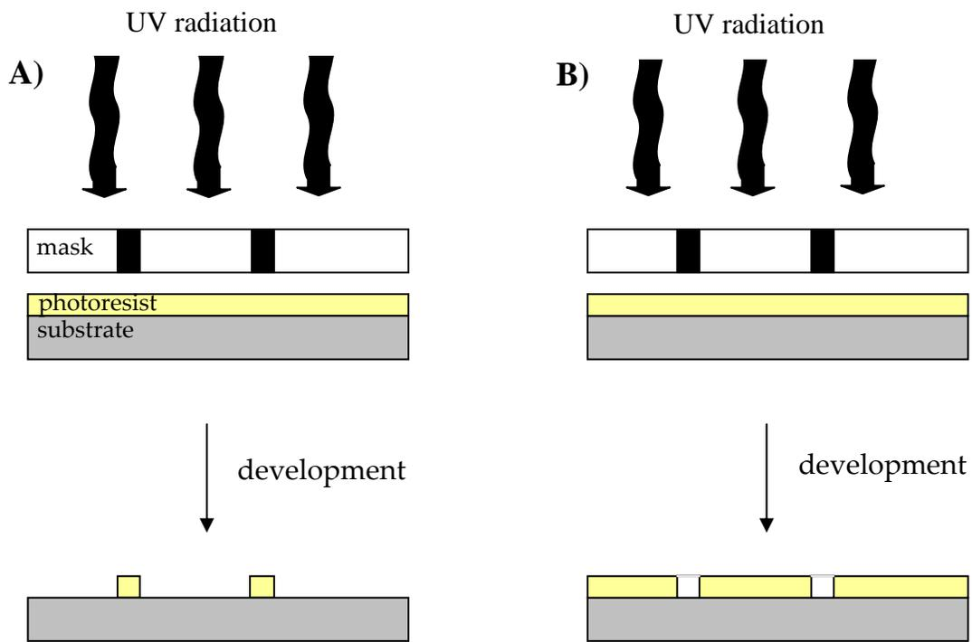
**Figure 1.2.** Effect of UV exposure and development on (A) positive and (B) negative photoresists.
