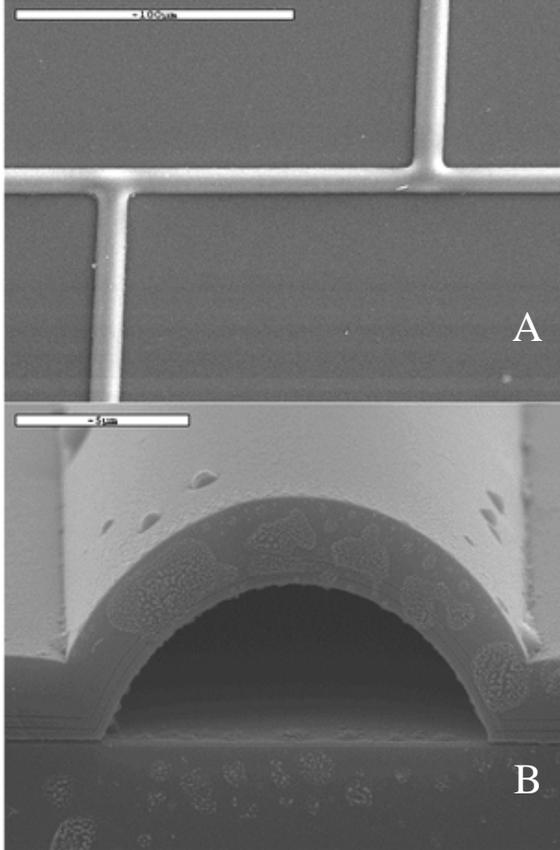
**Figure 2.3.** SEM images of an etched microfluidic tube made using the described procedure. (A) Top view of the offset injection region. (B) Profile view of the end of a channel.
