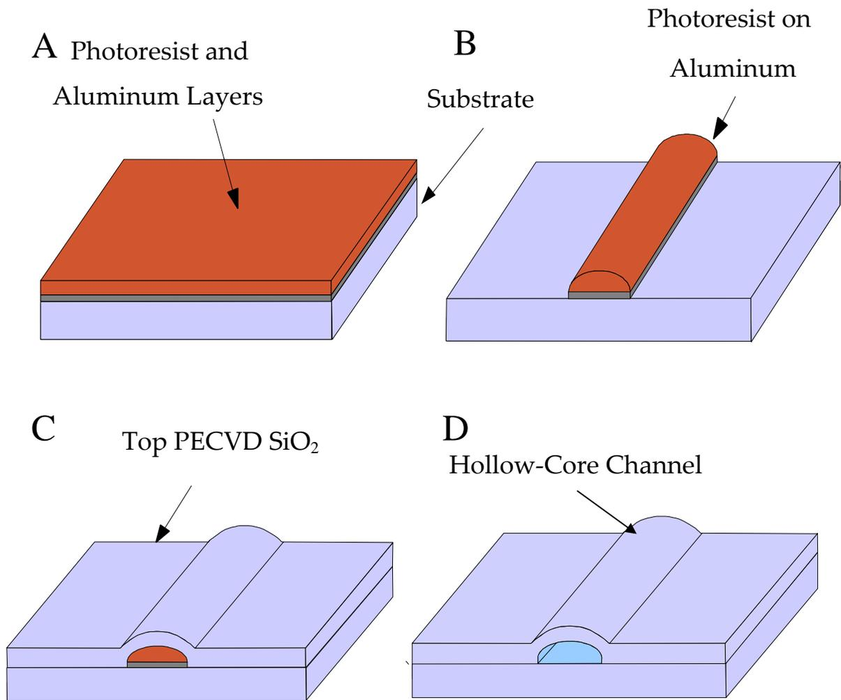
**Figure 2.1.** Schematic of the fabrication process for thin-film microfluidic devices. (A) Cleaned quartz substrate with 500 nm aluminum and 3  $\mu\text{m}$  photoresist. (B) Reflowed photoresist with etched aluminum sub-layer. (C) Patterned quartz wafer with 3  $\mu\text{m}$  oxide encapsulating the sacrificial layers. (D) Etched sacrificial layers forming a hollow tube.
