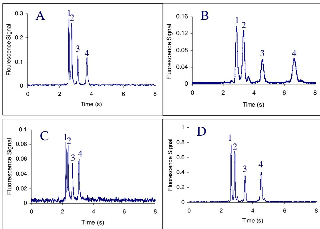
**Figure 3.1.** Electropherograms of the same mixture as in Figure 2.4. Coatings were Ultratrol Dynamic Pre-Coat HR in (A) and (C) and Ultratrol Dynamic Pre-Coat LN in (B) and (D). The electric fields for the separations were 660 V/cm in (A-B) and 830 V/cm in (C-D). Peaks are: (1) glycine, (2) phenylalanine, (3) FITC, and (4) arginine.
