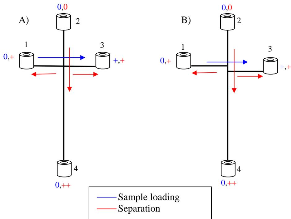
**Figure 1.1.** Schematics of general microdevice designs. Diagrams of (A) cross-channel and (B) double-T microfluidic device layouts. Sample loading is achieved by applying a voltage at reservoir 3 and grounding the others (1, 2 and 4). Injection and separation are achieved by rearranging the voltages such that the same voltage is applied to reservoirs 1 and 3, a larger voltage is applied at reservoir 4, and reservoir 2 is grounded.
