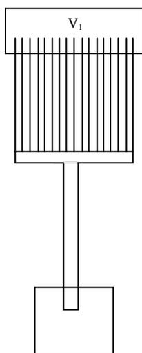
**Figure 4.3.** Thin-Film electroosmotic pump schematic.
