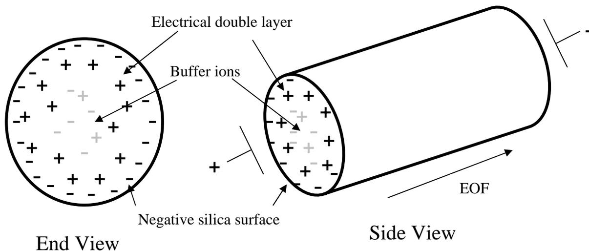
**Figure 1.3.** End and side view of the association between surface charge and buffer ions that gives rise to EOF in native SiO<sub>2</sub> columns.
