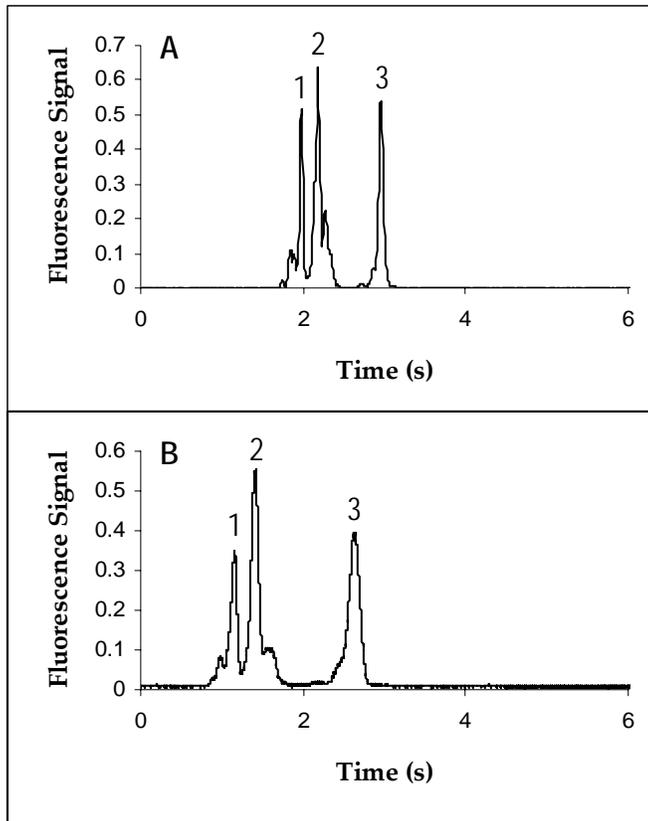
Figure 3.3. Separations of FITC-labeled (1) FLEEI, (2) Leu Enkephalin, and (3) GGYR in two different devices 6 months apart. (A) June 2005 and (B) December 2005. Separation potentials were 1250 V.
