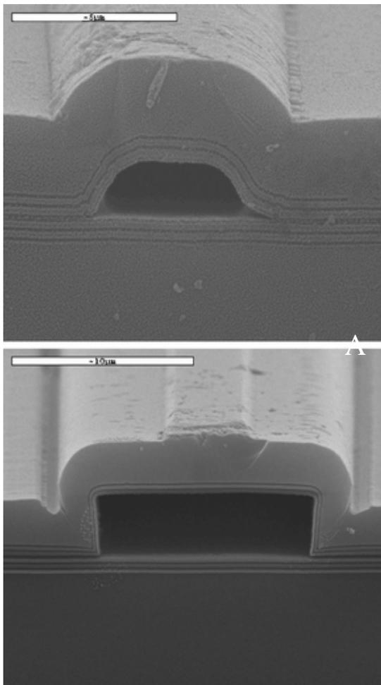
**Figure 2.5.** Profile SEM images of channels made using different sacrificial layers. (A) Channel made with aluminum sacrificial core, etched in 3:1 HCl/HNO<sub>3</sub>. (B) Channel made with SU-8 sacrificial core, etched in Nano-Strip.
