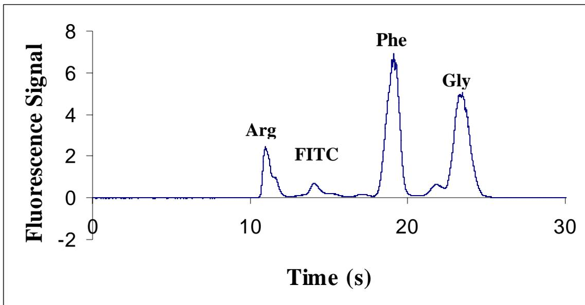
**Figure 2.4.** Electropherogram of FITC-tagged arginine, phenylalanine, and glycine. The injection concentrations were 500 nM of each amino acid.  $E_{\text{sep}}=580$  V/cm and  $L_{\text{sep}}=0.65$  cm.
