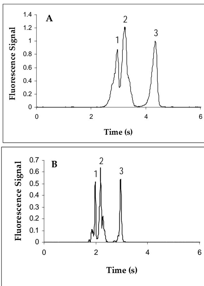
**Figure 3.2.** Separation of 3 FITC-labeled peptides using (A) 1000 V and (B) 1250 V in planar thin-film microfluidic channels using Ultratrol Dynamic Pre-Coat HR. Peaks are: (1) FLEEI, (2) Leu Enkephalin, and (3) GGYR.
