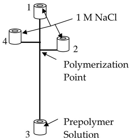
Figure 3.4. Schematic of the setup used to precisely define polyacrylamide gel interfaces in thin-film microfluidic devices.
