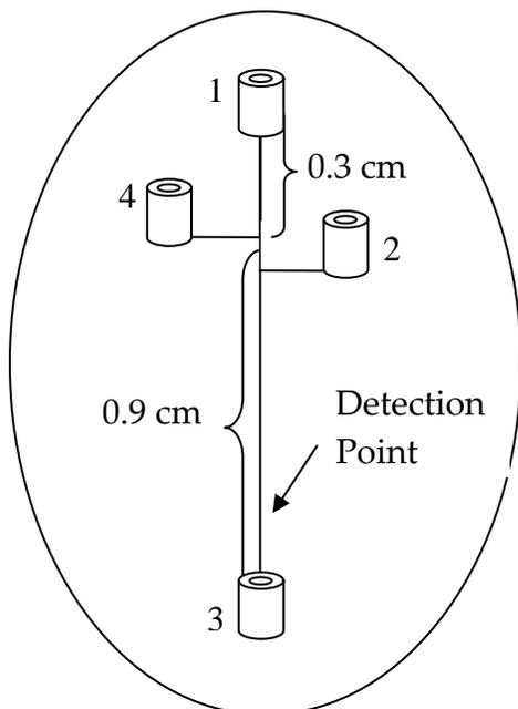
**Figure 2.2.** Schematic of the separation device layout. Reservoirs 1, 2, and 3 were filled with buffer solution, and reservoir 4 was filled with the amino acid sample. To inject, reservoirs 1, 3, and 4 were grounded and  $-600$  V was applied to reservoir 2. Separation was achieved by keeping reservoir 1 grounded, applying  $-600$  V to reservoirs 2 and 4 and applying  $-750$  V to reservoir 3. The offset of the double-T injector is not to scale.
