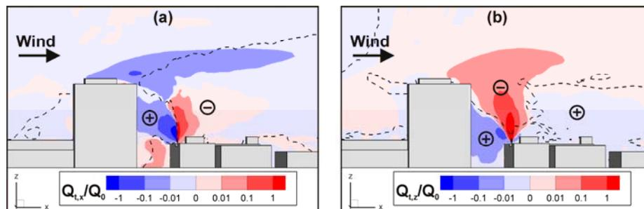
**Figure 6.** Case SW: Contours of non-dimensional turbulent mass flux components in the (a) streamwise and (b) vertical direction. The dashed lines represent the isolines  $\partial C/\partial x_i=0$  with (a)  $x_i=x$ , (b)  $x_i=z$ . The sign of  $\partial C/\partial x_i$  in the region delimited by the isoline is indicated in circles (+: positive; -: negative).
