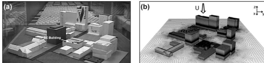
**Figure 3.** Case W: (a) wind-tunnel model and (b) corresponding computational grid on the building and ground surfaces (total number of cells: 5,257,343).
