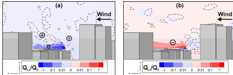
**Figure 8.** Case W: Contours of non-dimensional turbulent mass flux components in the (a) streamwise and (b) vertical direction. The dashed lines represent the isolines  $\partial C/\partial x_i=0$  with (a)  $x_i=x$ , (b)  $x_i=z$ . The sign of  $\partial C/\partial x_i$  in the region delimited by the isoline is indicated in circles (+: positive; -: negative).
