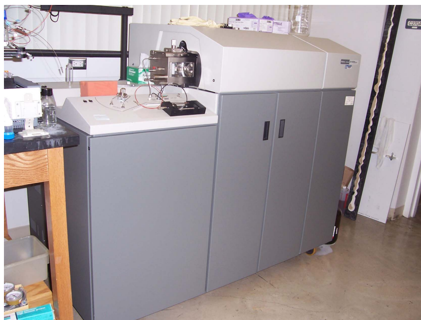
Figure 2.2: The Qstar Pulsar i ESI-LC TOF Mass Spectrometer used at BYU
