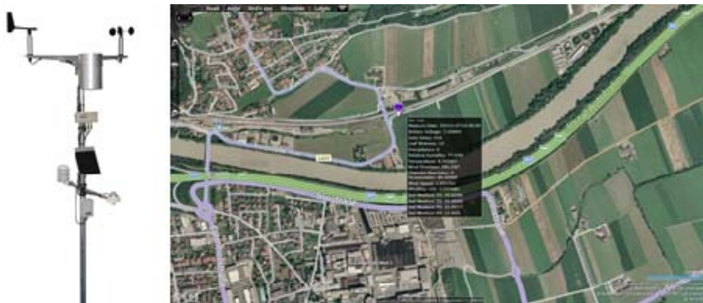
Abb. 6: Meteo-sensors with solar panel, com-unit and location on a map with data
