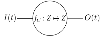
Figure 1: Structural view of a model component. The process representation f_C is encapsulated, while the inputs I and outputs O form the component interface.
