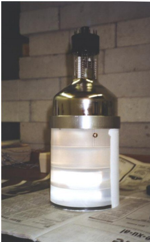
Figure 5. Detector, outside half-painted
