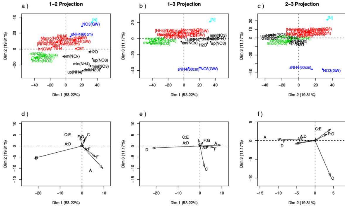
**Figure 4:** Principal Component Analysis and clustering of the results of the global sensitivity analysis of NitroScope. a - c ) projections of the clusters of outcomes onto the plane defined by two principal components; d - f ) projections of sensitivity indexes of input factors onto the plane defined by the principal components.
