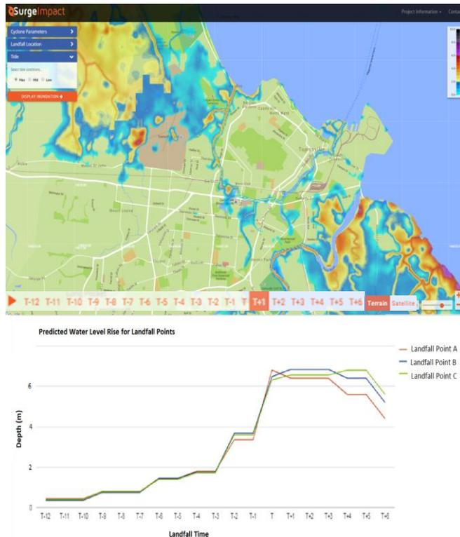
**Figure 3.** Water depth in Townsville (top) and Delivery report from SurgelImpact for a Tropical cyclone category 5 making landfall 60 km north of Townsville with a RMW =40km, forward Speed =10 m/s and hitting the coast with a 200 °N direction (bottom).
