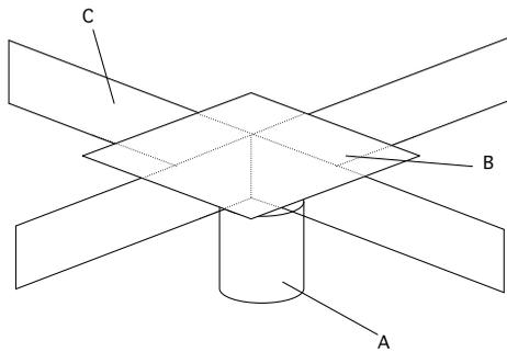
Fig. 1. Schematic of pitfall trap: A, trap receptacle; B, cover; C, baffle.
