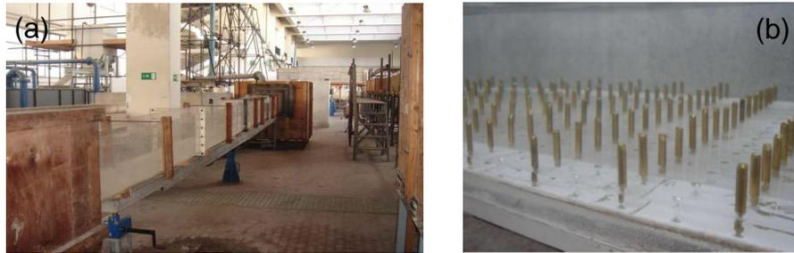
**Figure 2.** (a) Channel and (b) vegetated bed.
