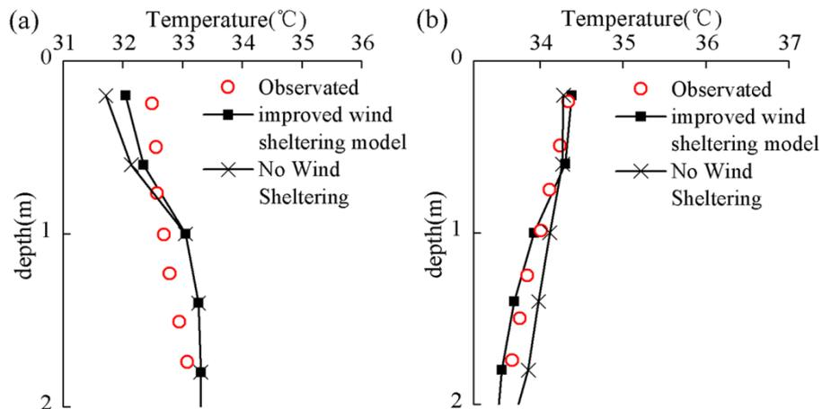
**Figure 6.** The comparison of the simulated and the observed vertical water temperature on July 14, (a)8:00am; (b)5:00pm.
