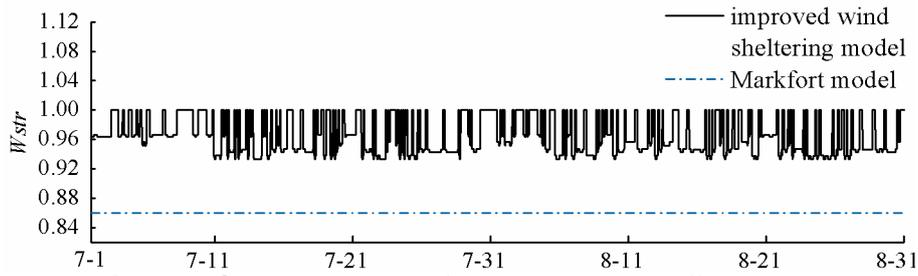
Figure 4. Calculation result of wind sheltering coefficient  $W_{str}$ .
