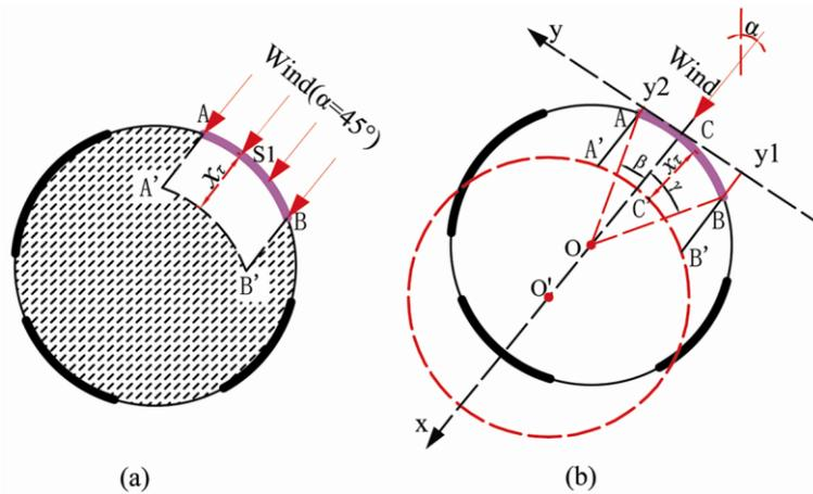
Figure 2. Geometric schematic of wind sheltering effect.
