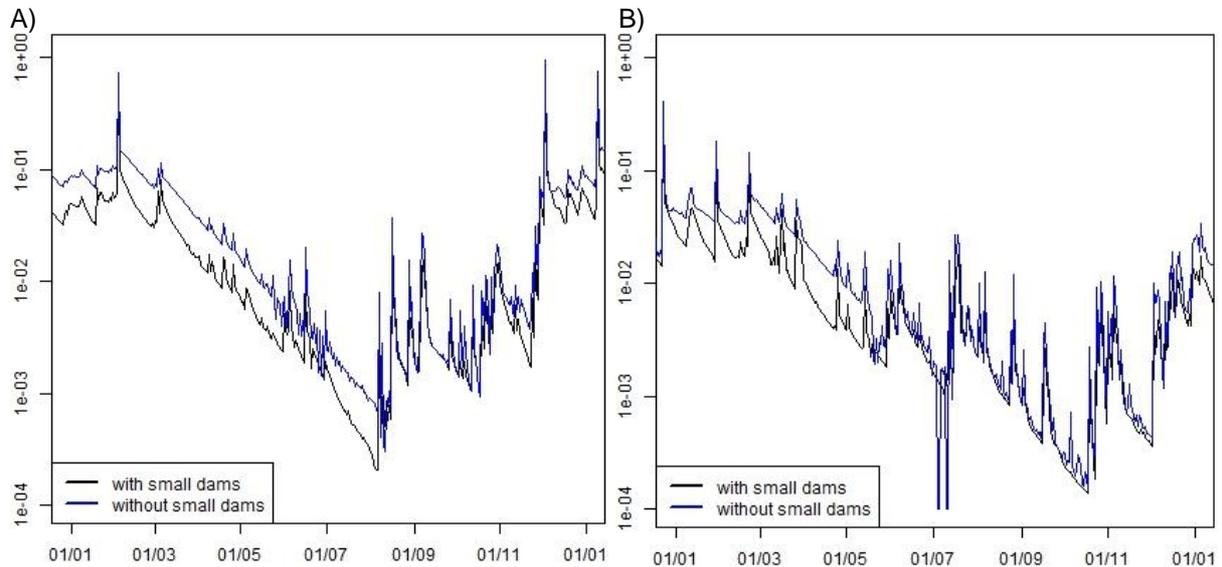
**Figure 2.** Comparison of water flow ( $\text{m}^3/\text{s}$ ) for a selected watershed of the Aveyron river basin (minimum flow of SWAT sub-watershed of the selected area) in A) 2003 and B) 2011. The black line represents the simulation with small agricultural dams and the blue line the simulation without dams.
