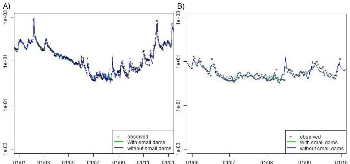
**Figure 1.** Comparison of water flow ( $m^3/s$ ) at Loubejac (the outlet of the Aveyron basin) between observations (black stars), simulation with small agricultural dams (green line) or without dams (blue line) for respectively A) the full year 2003 or B) the low water period (June-October) 2003.
