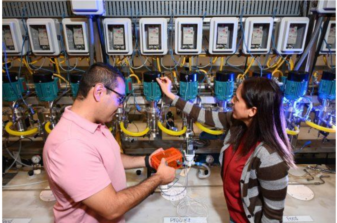
Figure 1: Example of solvent extraction equipment, like that used in the Beartooth physical system, though without a glovebox. Image from https://inl.gov/integrated-fuel-cycle-solutions/
