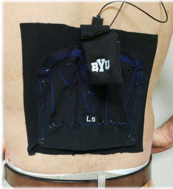
Figure 1: Brigham Young University's SPINE Sense System, applied to the lower back of a researcher
