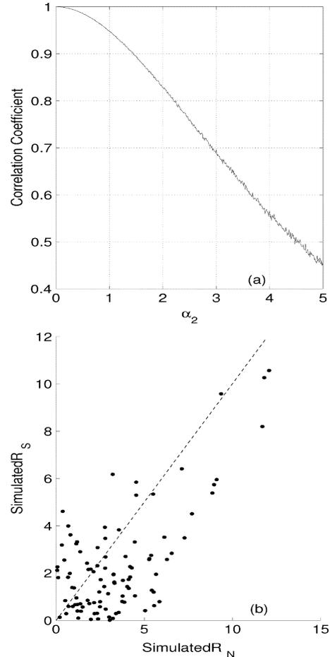
Fig. 11. Monte Carlo simulation result for the simple SeaWinds/NEXRAD noise model. (a) Shows  $\alpha_2$  versus correlation coefficient for the additive noise Monte Carlo simulation. Correlation nears 0.75 when  $\alpha_2$  is 2.5. (b) Displays the scatter plot created simulation at  $\alpha_2 = 2.5$ .
