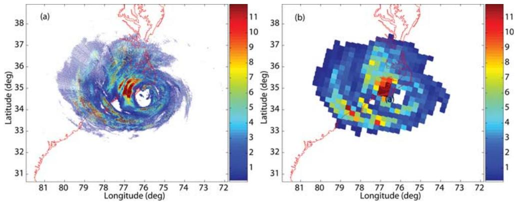
Fig. 1. Rain rate data from the Moorehead City, NC NEXRAD installation averaged into (a)  $1 \text{ km} \times 1 \text{ km}$  and (b) SeaWinds  $25 \text{ km} \times 25 \text{ km}$  WVC-sized vertical bins from Hurricane Isabel's landfall (September 18, 2003, 16:00 UTC) displayed on a latitude/longitude grid.
