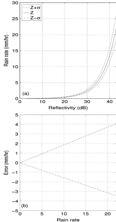
Fig. 9. (a) NEXRAD rain rate versus reflectivity. Rain rate is plotted as a function of  $Z$  with  $\pm\sigma$  envelopes. The solid line is the nominal  $Z$ - $R$  relationship, and the dotted lines show the relationship when  $Z = Z \pm \sigma$  where  $\sigma = 1$  dB. (b) Differences between calculated and true rain rate for  $Z \pm \sigma$ . The standard deviation of the rain rate estimation is approximately  $0.2R$ , where  $R$  is the true rain rate.
