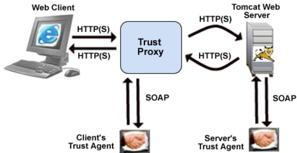
**Figure 1: Architecture for Trust Negotiation**
