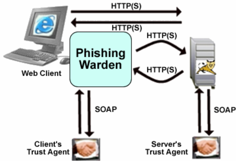
Figure 5: Model of trust negotiation without a proxy by using the browser plug-in Phishing Warden
