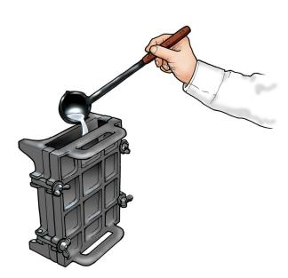
3 Molten metal is now poured into the tightened frame to create a precise cast of the original typeset form. When the metal cools, the resulting stereotype is used in the press just like the original typeset form.
