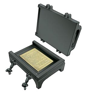
2 When the flong has dried, it is placed into a hollow metal frame and covered with a lid. The frame is then screwed tightly together and tilted up vertically.
