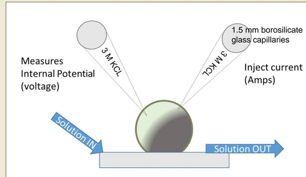
**Fig. 1.** Representation of two-electrode whole cell voltage clamp. We used a pressurized perfusion system that quickly changes the solution applied to the oocyte.
