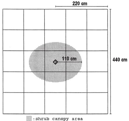
Fig. 2. Depiction of sampling grid for small-scale spatial heterogeneity work. Sampling points were established at each line intersection ( $n = 36$  points per shrub). Samples were collected at 2 depths (0–7.5 cm and 7.5–15 cm) for a total of 72 samples per shrub. This figure depicts an example shrub that measures 110 cm across.
