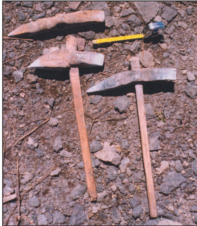
Figure 4.6. Chisels used by metateros during the roughing-out of manos and metates in the quarries.
