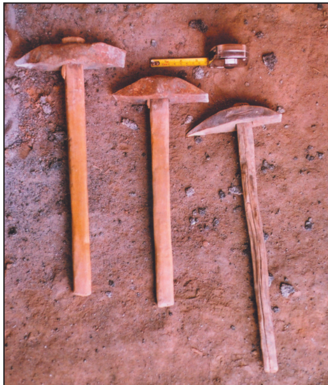
Figure 4.8. Chisels used by Jacinto Guachiac Sohom during the finishing of manos and metates.
