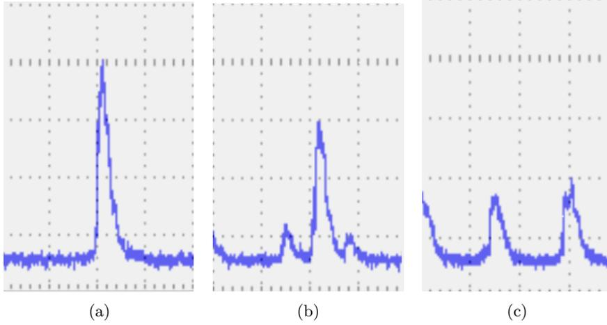
Figure 1: **Spectral Output of Slave Laser While Injection Locked.** *Horizontal scale is in 20mV increments. a) Stable injection lock. The peaks are tall and narrow. b) Still injection locked but side bands have appeared. c) Still interacting with the master laser but the side bands have taken over and the main frequency is no long clear. As the strength of the injection lock decreases, so does the height of the main peak.*
