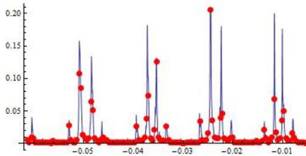
Figure 2: **Digitally Finding Peak Values.** *Finding the peak value is limited by the sampling rate and the narrow width of the peaks. The likelihood of any particular data point measuring the peak voltage is proportional to the width of the peak over the width of a complete scan (i.e. the width before it repeats itself).*
