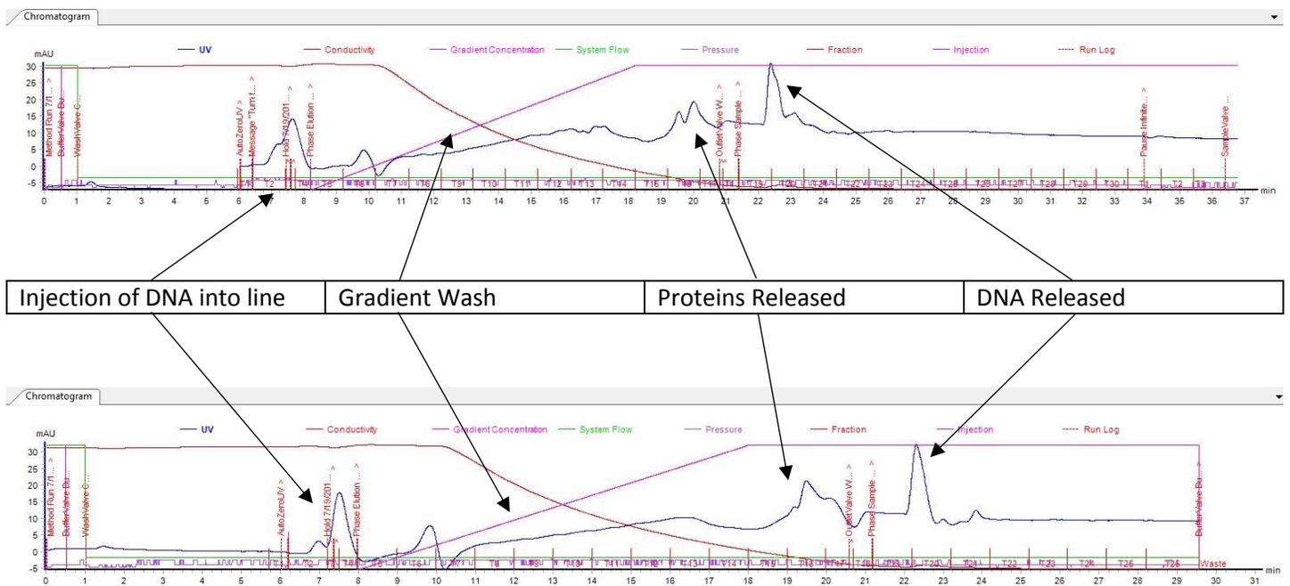
Image 12: Chromatograms produced by the AKTA Chromatograph and Unicorn One Software for tests 5.1.3 and 5.1.4.
