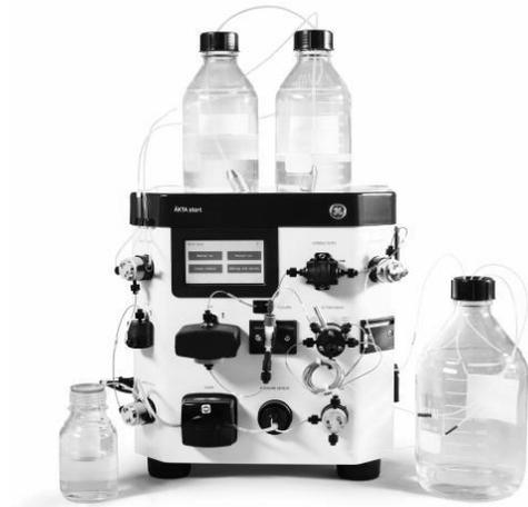
Image 3: AKTA Start Chromatograph used for precise monitoring of the flow rates, column volumes and number of mL of each buffer used [5].
