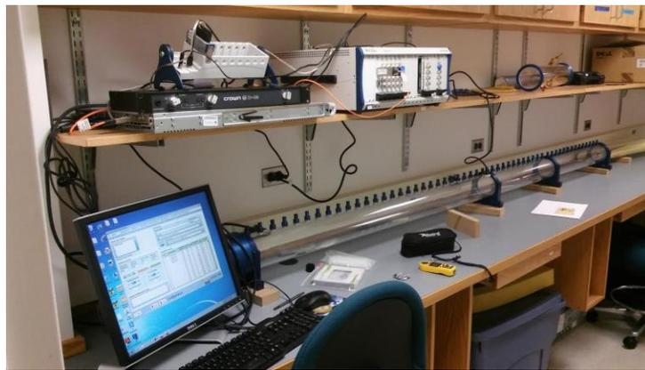
*Figure 1. Photograph of the plane-wave tube and data-acquisition system.*
