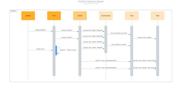
Figure 2: Sequence Diagram of the Terraform Script. From left to right: Variables, VPCs, Subnets, Security Groups, Hosts, and Tasks.
