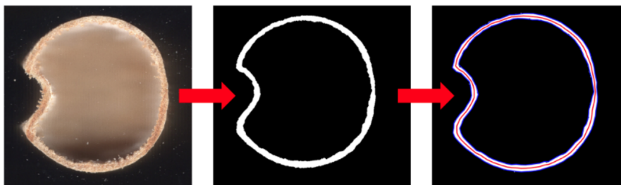
Figure 3.4: Three steps of the image segmentation process. We first imported an image to Matlab (left), then we separated the rind pixels from the pith pixels using the segmenter tool (middle), then relevant quantities were calculated using Matlab functions (right).
