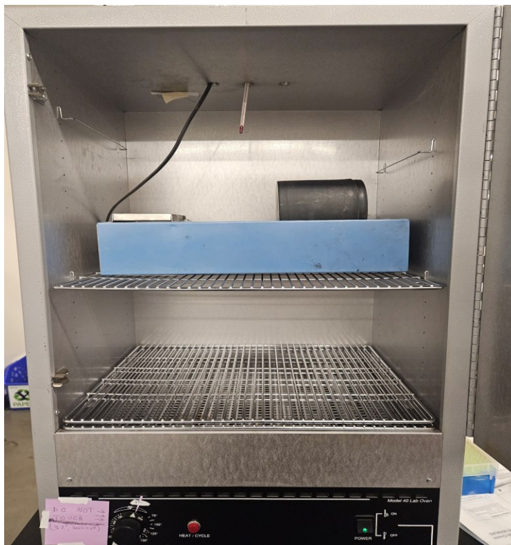
Figure 17: Drug release convection and temperature control setup. Vials are contained in a cylinder (black) placed on a rotating frame (blue) within an oven.
