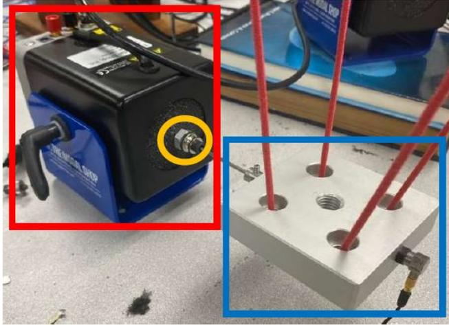
Figure 3.3: Shaker Body (Red), Armature (Orange), and Calibration Mass (Blue)
