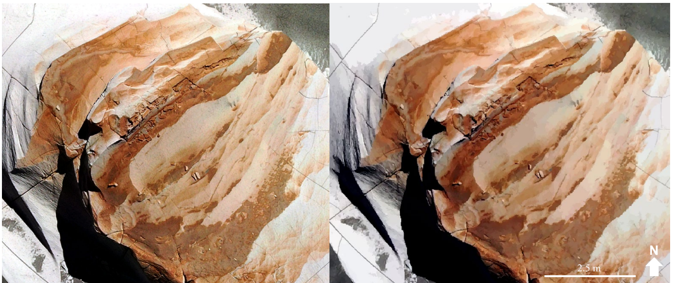
Figure 13; Zoomed in orthomosaic of a yardang (left) and segmented image, where similar pixel colors are grouped together (right).
