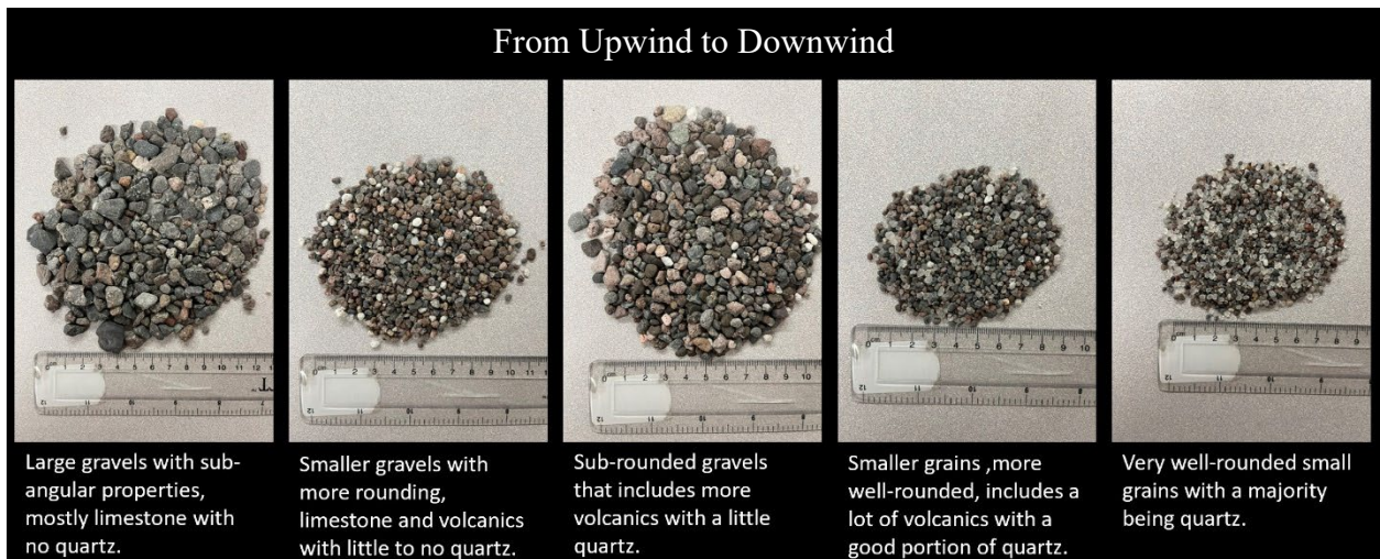
Figure 26; Gravel sample results from upwind to downwind with a description of size, shape, sorting and composition below the images.
