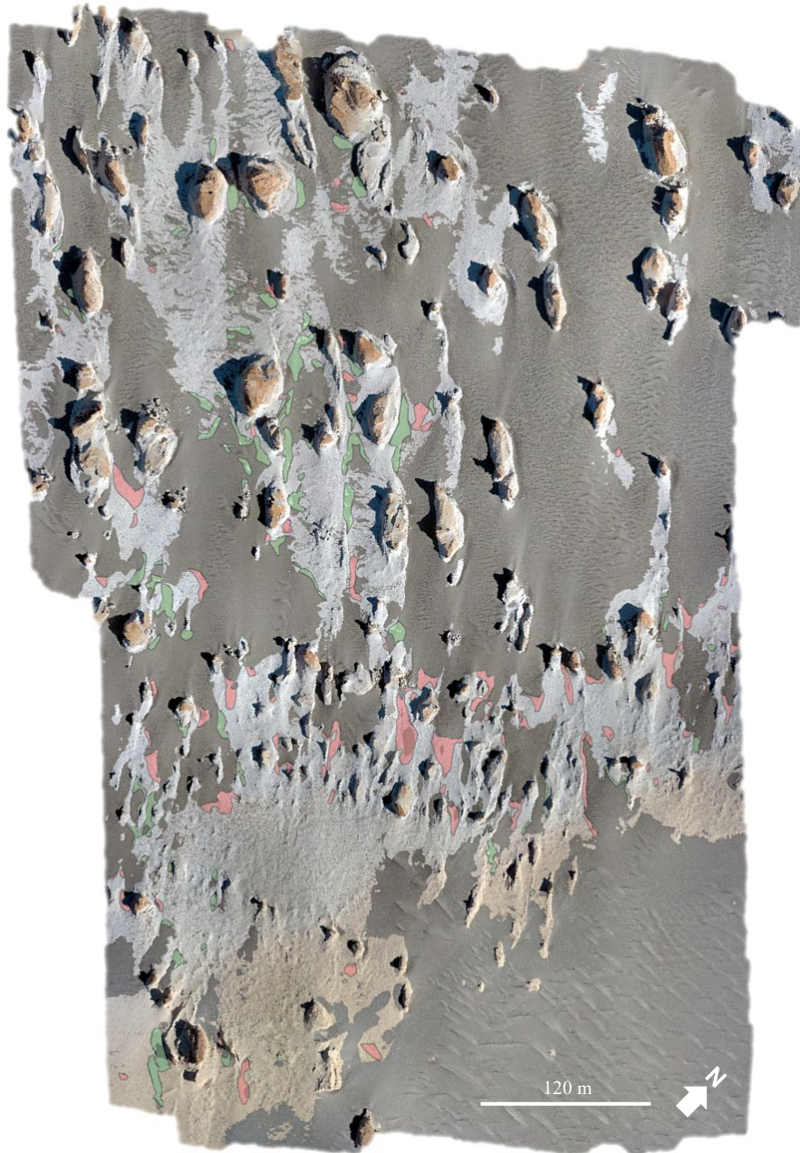
Figure 24; Orthomosaic from 2024 showing areas (green) where there was no gravel in 2019 but is currently present and areas (red) where there was gravel in 2019 but is not currently present.
