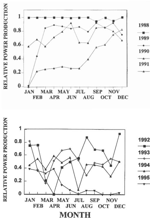
Fig. 2. Relative monthly power production for 1988–1995 at Wabuska Geothermal Plant, Nevada. Monthly production was scored relative to the highest observed amount of power produced during that particular month. For instance, the highest production during January was observed in 1988; all other January production values were scored relative to this score.
