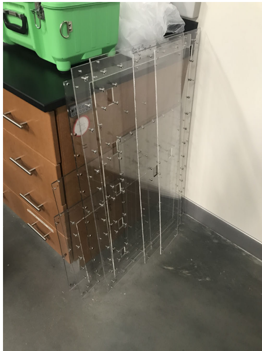
Figure 5.11: Acrylic pieces after epoxying the 1/4-20 screws and half of the 6/32 screws.
