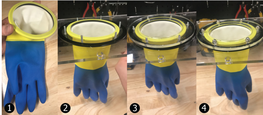
Figure 5.18: Process for assembling the glove door. (1) Wrap the glove around the small ring. (2) Place the small and large rings on the door. (3) Place the top ring over the bottom rings. (4) Bolt the ring using acorn nuts.
