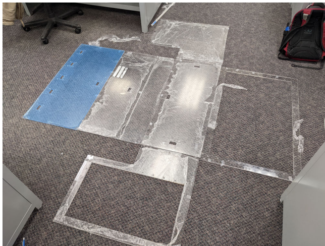
Figure 5.5: Main acrylic pieces after being laser cut and tapped.
