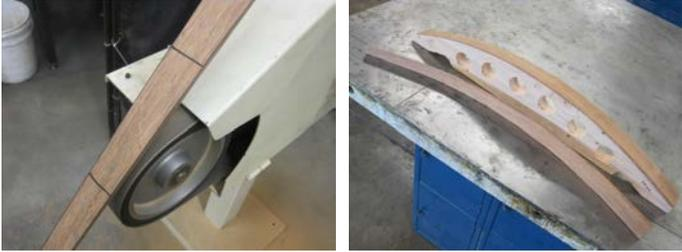
(c) Tapering thickness with a belt sander (d) After applying heat, the bamboo core is bent to its final shape.
