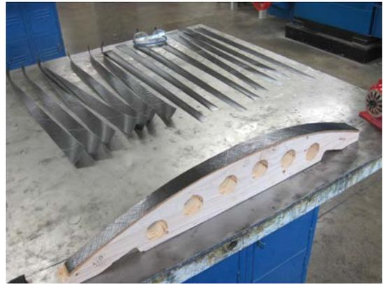
Figure 7: A layup in progress. One woven ply has been applied to the core; the others wait in the background.
