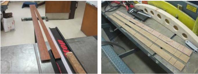
(a) Trimming the flooring material (b) Bamboo blanks with width reduced
