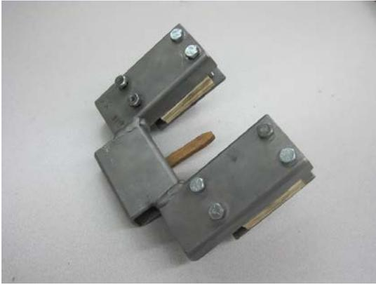
Figure 9: Steel handle with wooden soft jaws and bamboo arrow rest.
