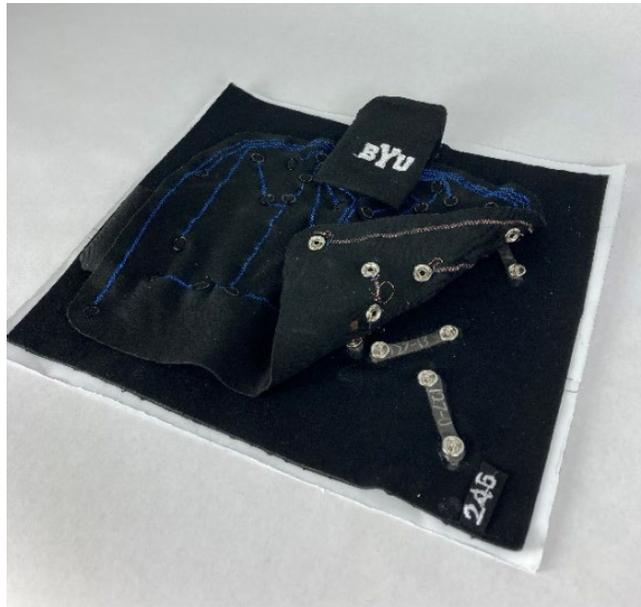
Figure 5.5 The vertebral motion tracking system of 16 nanocomposite sensors (two are visible from underneath the cover in the lower right side) on kinesiology tape with stitched wiring.
