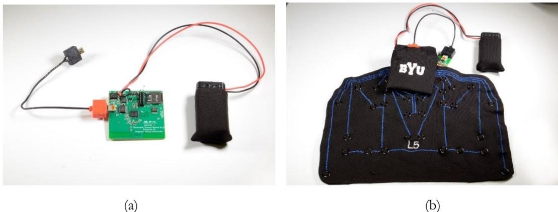
Figure 5.6 (a) Custom PCB for reading the resistance across all 16 piezoresistive sensors and (b) integration of PCB with final SPINE Sensor System.
