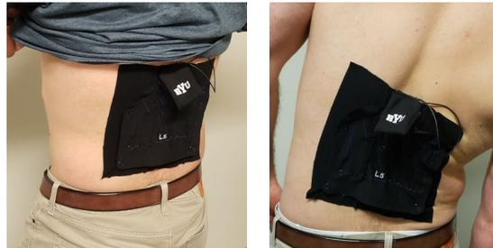
Figure 6.2 Depiction of (a) the SPINE Sense System adhered to a subject’s back and (b) the SPINE Sense System collecting data during motion.
