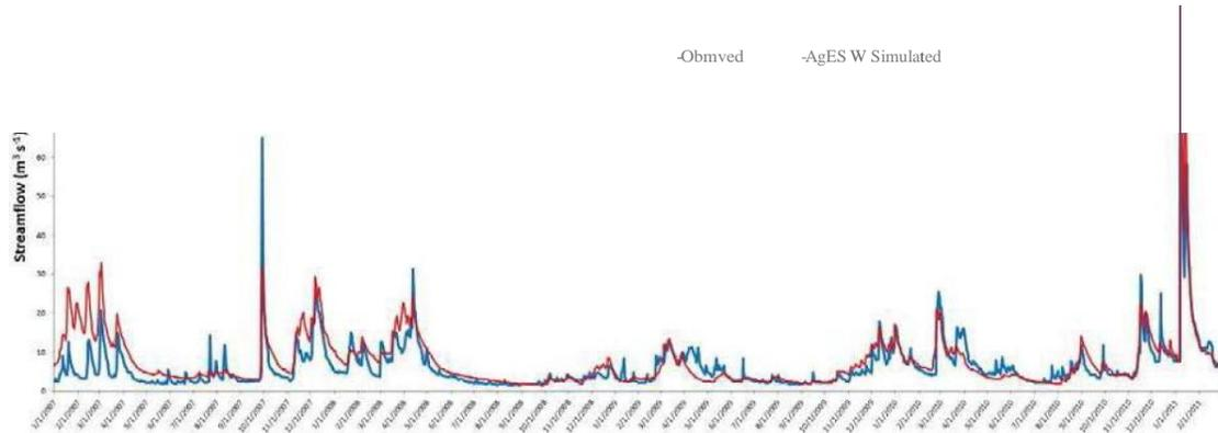
Figure 2. Daily Upper Gera Watershed AgES-W simulated and observed streamflow ( $\text{m}^3 \text{s}^{-1}$ ) at the Moebisburg gauge (validation period -1/1/2007 to 6/30/2012).
