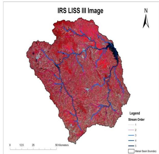
Fig: 5 Extracted Drainage Network overlaid on IRS LISS III Satellite Imagery of Manair Basin
