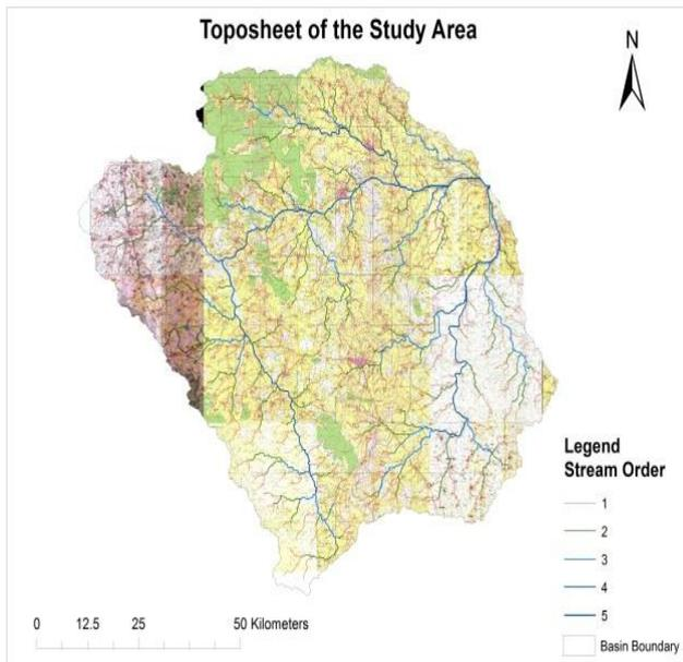
Fig: 4 Extracted Drainage Network overlaid on Toposheets for Verification of Manair Basin
