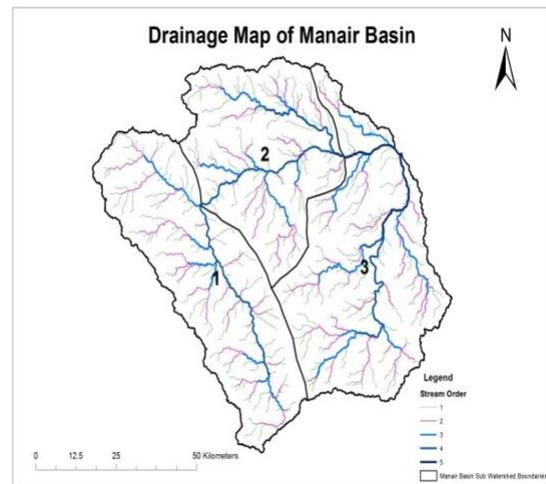
Fig: 3. Extracted Drainage Network and Sub-Watersheds 1-Upper Manair, 2-Mid Manair & 3-Lower Manair from delineated DEM data of Manair Basin
