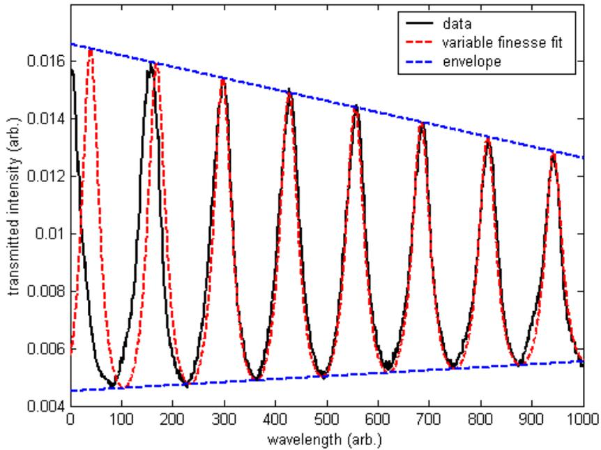
**Fig. 18.** Comparison of FP transmission with a fit having finesse that varies according to the trendline shown in Fig. 17 and bound by the envelope shown. The fit assumes that the period is constant and that changes in the measurements of finesse are due entirely to changes in peak width. This appears to be a reasonable assumption everywhere except at the first two peaks, where the increased period is obviously responsible for the higher finesse.
