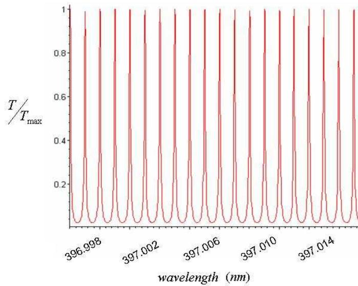
**Fig. 2a.** Low finesse cavity transmission with peak width of 190MHz. The mirror separation would have to be 7.9cm to achieve this signal using a parallel plane FP cavity.
