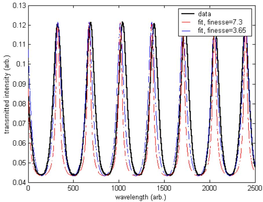
**Fig. 14.** Transmission of the nonconfocal cavity with mirror separation of 80cm and infrared input compared with predicted signals for coherent and incoherent input. The larger finesse corresponds to coherent input.
