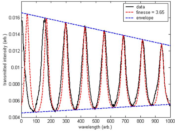
**Fig. 16.** Transmission of the confocal cavity compared to the transmission predicted when taking the attenuation into account.
