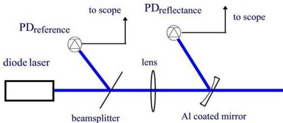
**Fig. 11.** Set-up for measuring mirror reflectivity.
