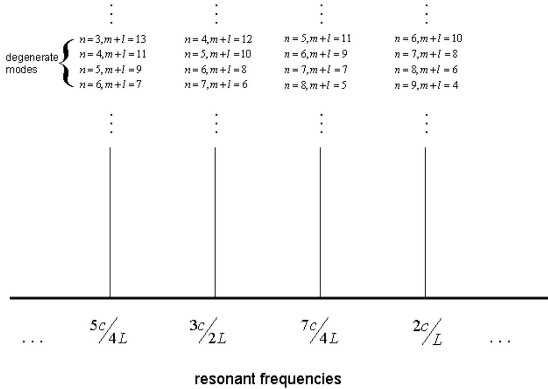
**Fig. 4.** Degeneracy of modes in the confocal cavity. Nearly all modes are degenerate with other modes having either odd or even values of  $m + l$ .
