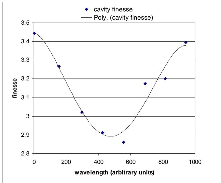
**Fig. 17.** Measured cavity finesse vs. wavelength. The trendline, a 4<sup>th</sup> order polynomial fit generated in Microsoft Excel, was used to generate the variable finesse fit for the transmission shown in Fig. 16.
