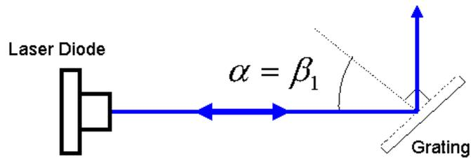
**Fig. 8.** Diffraction grating in Littrow configuration. The first-order beam is diffracted back into the diode for amplification of the selected wavelength.
