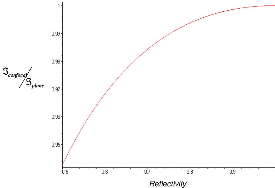
**Fig. 7.** Ratio of the confocal to the plane cavity finesse. The two are nearly equivalent, even for 50% reflectivity. As mirror reflectivity approaches 1, the two finesesses approach exact equality.
