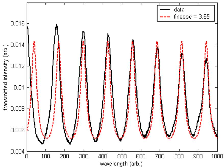
**Fig. 15.** Comparison of confocal cavity transmission with the signal expected for spatial incoherence and/or off-axis propagation
