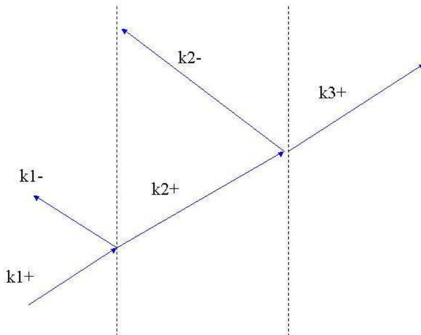
**Fig. 1. Plane wave propagation vectors in the double boundary problem. Note that angles from normal are grossly exaggerated. Adapted from [2].**
