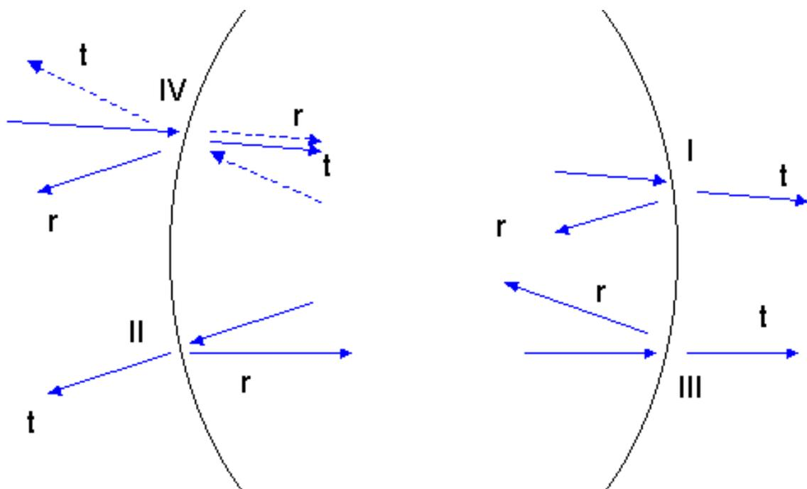
**Fig. 6.** Re-entrant rays in a confocal cavity. The dashed line indicates the second interaction at *IV*. At each reflection, the electric field amplitude is multiplied by  $r$ . The electric field transmitted at *I* is a superposition of all rays that exit after 4, 8, 12, . . . reflections. Adapted from [1].
