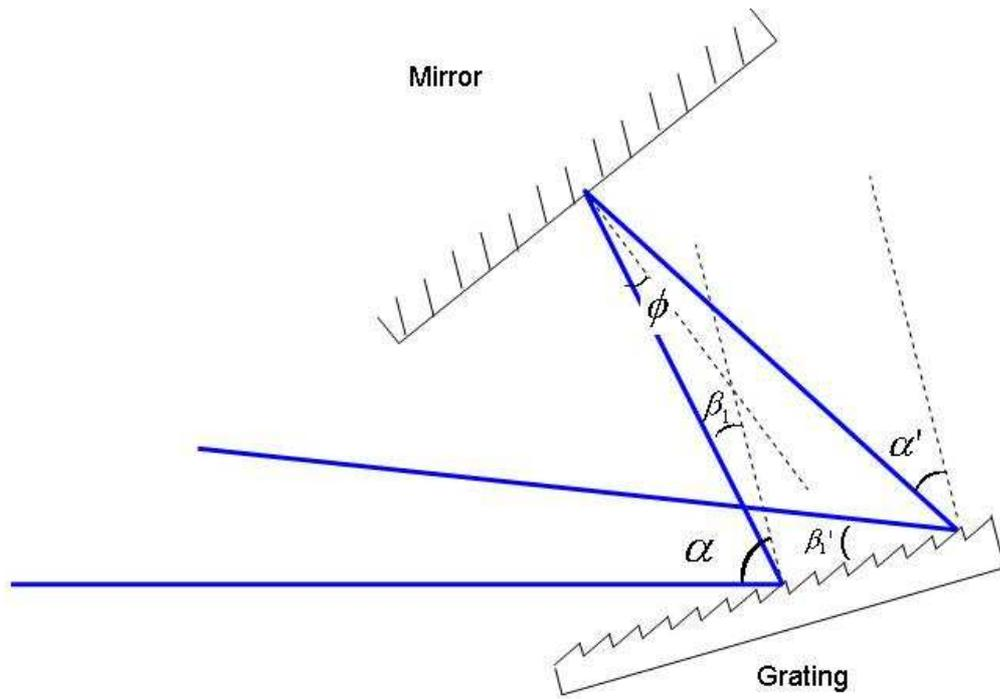
**Fig. 10.** Alignment in Littman-Metcalf configuration. The angle  $\phi$  must be zero in order that  $\alpha = \beta_1'$ . Adapted from [8].
