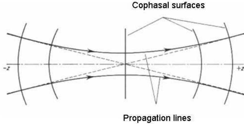
**Fig. 5.** Gaussian beam propagation in a confocal cavity. The beam waist is located in the center of the cavity, and the radius of curvature is matched to the curvature of the mirrors. Reproduced from [1].
