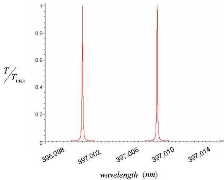
**Fig. 2b.** High finesse cavity transmission with the same peak width as in Fig. 2a. This signal may be obtained with a parallel plane cavity with a mirror spacing of 1.0cm.
