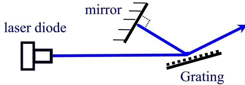
**Fig. 9.** The Littman-Metcalf external cavity. The condition for feedback requires that the first order beam strike the mirror at normal incidence. Its principal advantage is that the output beam does not change direction with tuning. Tuning is accomplished by changing the mirror angle slightly.
