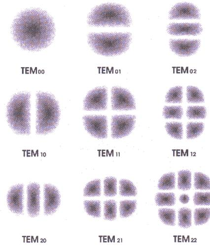
**Fig. 3.** Spatial mode intensity patterns. The first and second subscript digits indicate the number of nodes on the horizontal and vertical axes respectively. Nodes are manifest as minima in the intensity. Reproduced from [4].
