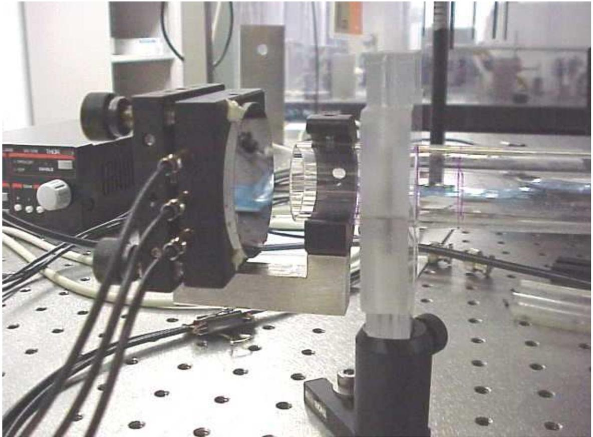
**Fig. 12.** One end of the Fabry-Perot cavity.
