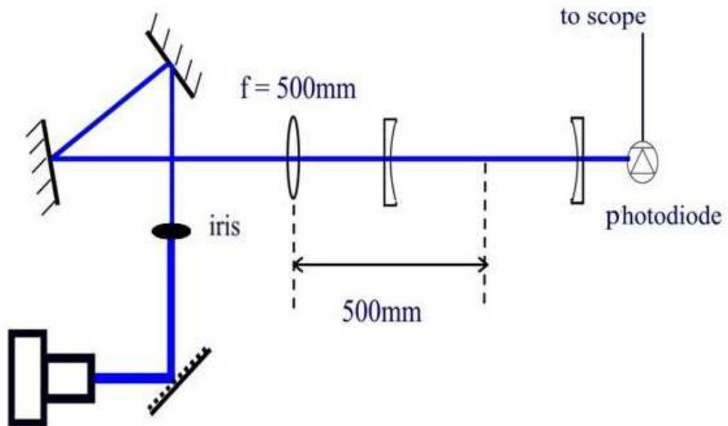
**Fig. 13.** Experimental set-up used to test the Fabry-Perot cavity.
