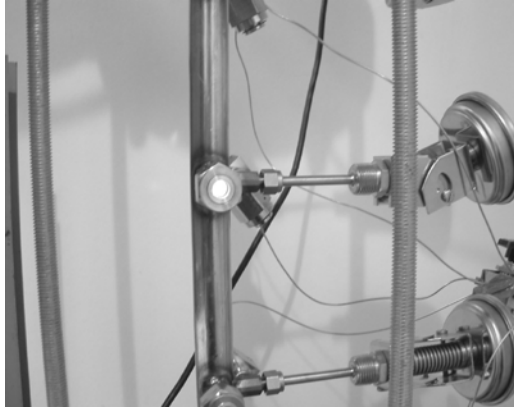
Figure 3. Corona discharge as seen through a viewport
