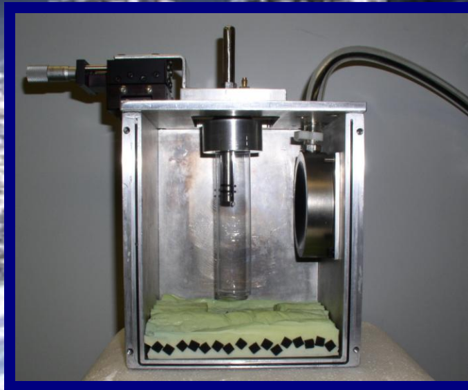
Figure 6. This is a photograph of the sonication chamber. The transducer is on the right while the pressurized chamber and sample holding rod are located in the center.
