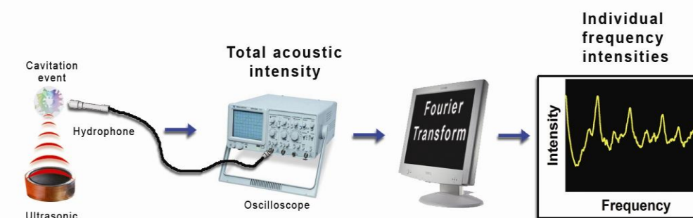
Figure 5. Hydrophone readings of fluorescence experiments were converted from time to frequency domain (Fourier Transform), thus generating acoustic spectra that describe the bubble vibrations at individual frequencies.
