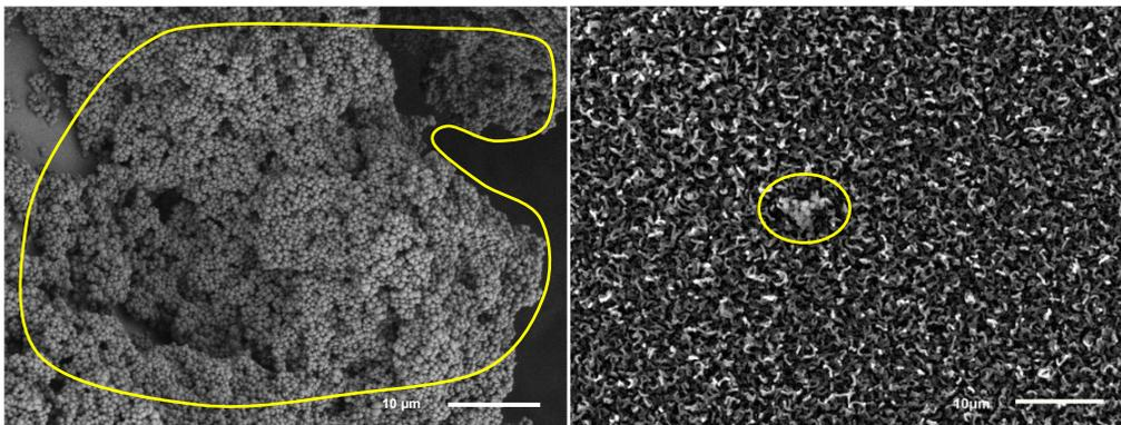
**Figure 1:** Comparison of standard MRSA growth on a PEEK surface to growth on a CICNT coated silicon wafer. Areas inside the yellow shapes show MRSA growth. Reference scale is 10 µm.
