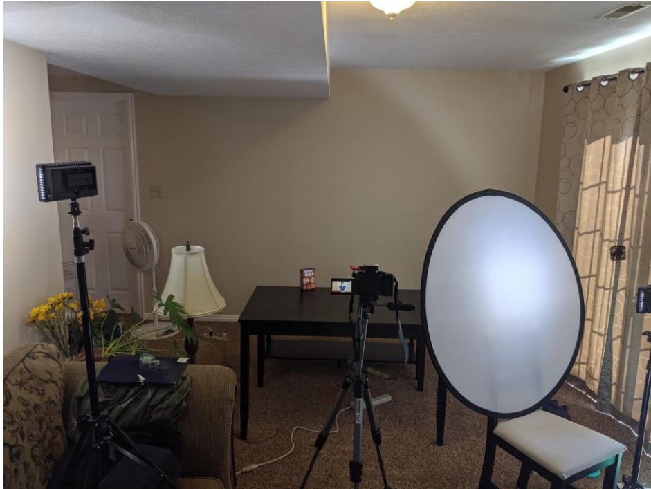
Figure 47. Current film setup. Table in middle of room with seating for host behind. 2 LED lights at right and left, each on a light stand. Diffuser disc in front of the right light, and the left light reflects off the white wall. Camera directly faces table, host, and plain wall (This position is used for wide shots. Close-ups have the camera closer to the table). Wireless microphone receiver is attached at top of camera.
