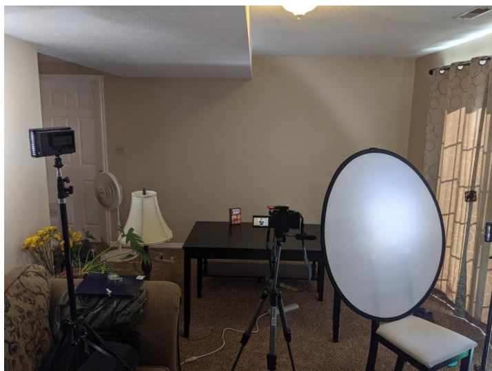
Figure 5. Current film setup. Table in middle of room with seating for host behind. 2 LED lights at right and left, each on a light stand. Diffuser disc in front of the right light, and the left light reflects off the white wall. Camera directly faces table, host, and plain wall (This position is used for wide shots. Close-ups have the camera closer to the table, or leaning against it). Wireless microphone receiver is attached at top of camera.
