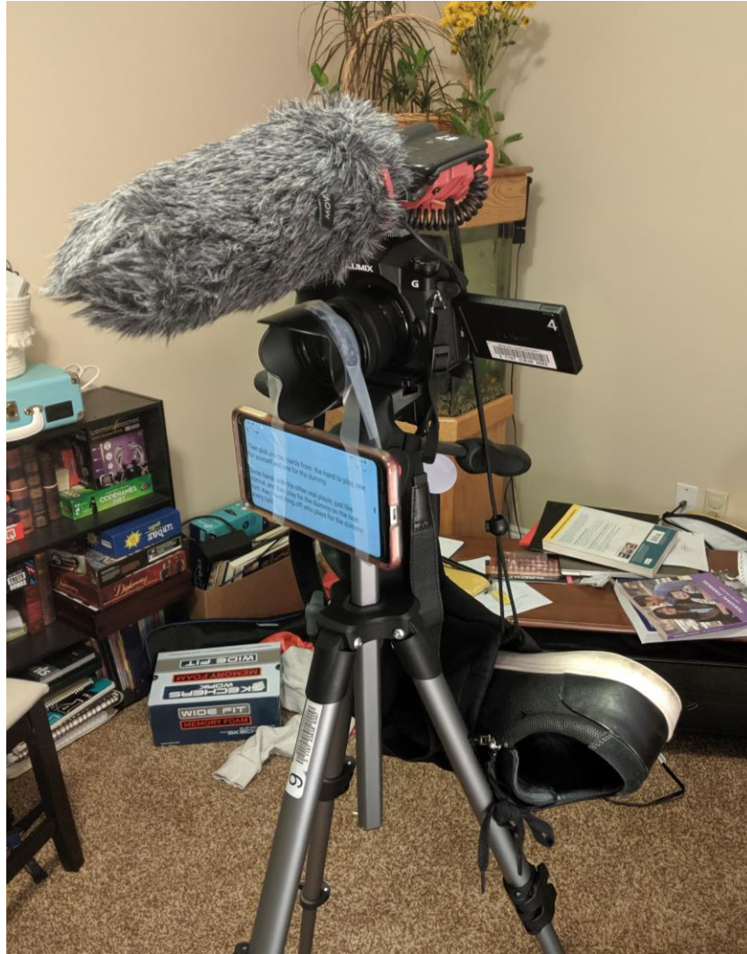
Figure 50. An improvised weight used to keep the shotgun mic out of frame.
