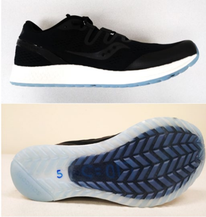
Figure 1. Stiff Plate Placement in Training Shoe A carbon fiber plate was inserted between the midsole and outsole of a Saucony Freedom shoe. The bottom image shows placement of this plate, covering the forefoot but not extending all the way to the heel.
