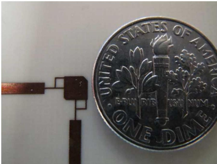
Figure 3.5: Fabricated antenna closeup. Despite its small size, the antenna's features can be accurately fabricated using standard etching techniques.
