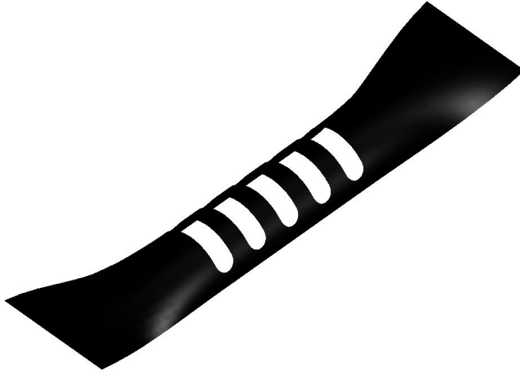
Figure 2.12: The Torsional U-form Flexure.
