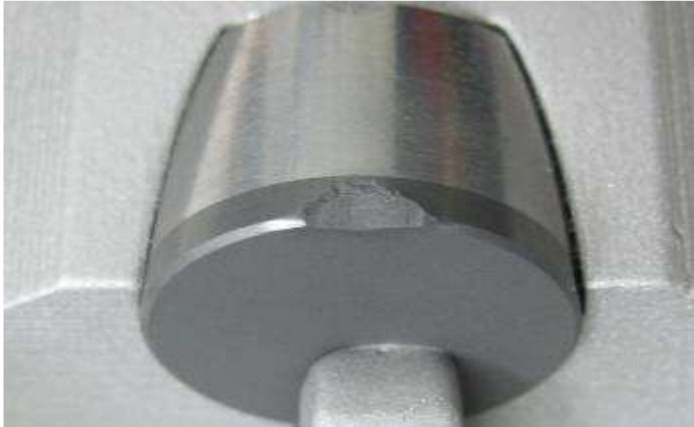
Figure 4-1: Polycrystalline diamond compact inserts after 50 passes on the wet VTL test.
