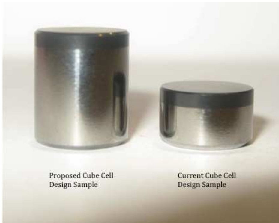
Figure 3-4: Proposed method finished sample compared to current method finished sample without bonding process.
