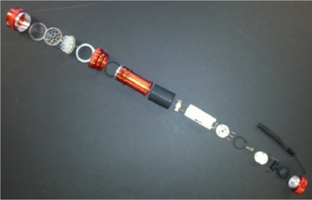
Figure 6: Exploded View of Entire Original Flashlight (Orange Version)
